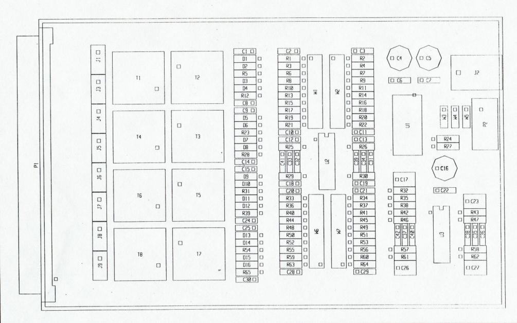
LAYOUT NOTE. MARKED PIN ON LAYOUT DENOTES FOR LEDS: CATODE PIN ,SHORT PIN OR PHASED BODY SIDE DIODES: CATODE PIN TANTAL AND ELECTROLYT: POSITIVE PIN CONNECTORS. LA OR AL PIN
