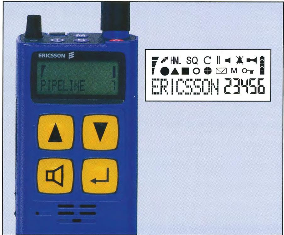
his primary tasks. An example of this is the convenient location of the volume knob on the top of the station. Here you will also find the on/off switch and an emergency alarm button.
